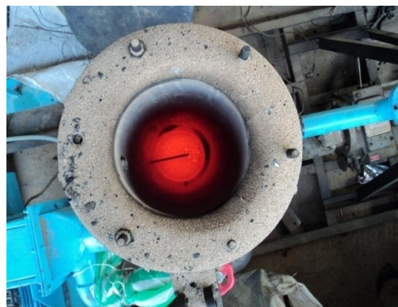
Fig. 22: a and b [12] a) Side view of BFBC, the upper section could be seen at the background b) An aerial view of the BFBC during one of the experimental runs. Elutriated particles could be seen on the flange of the lower section. Inert bed temperature at this point was 801°C. The dark straight line on top of the bed was the third thermocouple (temp. 627 °C). The incorporated partitioning of the combustor body into lower section and upper section makes this view possible.
